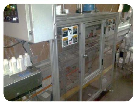
The desired result for the bottle entering the in-feed is for the belt groove in the bottle dome to be level with the belt. This will allow a smooth transition when the bottle enters the pickup point of belts.
