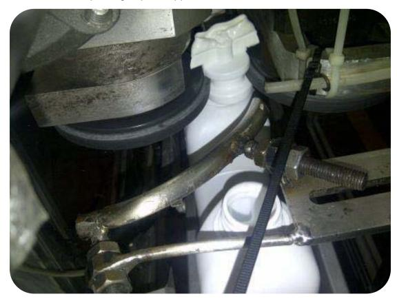
New Trimmer has bracket system that will need to be welded.
